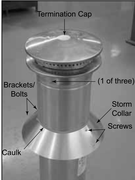
Figure 10.19 Install Vertical Termination Cap
